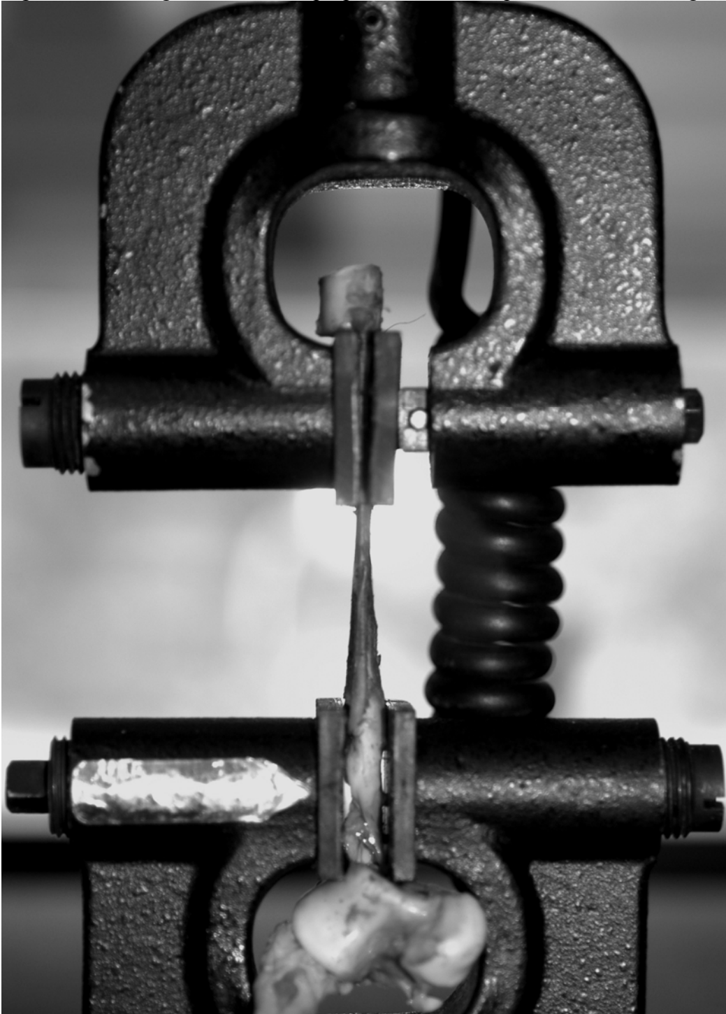
Figure 5.6. Mounting protocol to test the material properties of the posterior tibiotalar ligament (PTTL). Proximally, the bone-ligament-bone complex is clamped into the Instron apparatus and resists slipping downward by the T-shaped cortical bone. Distally, the tibia is cut along the medial malleolus such that it and the posterior tibiotalar ligament can fit between the Instron clamps without interference. The bone-ligament-bone complex is held in place distally by the superior and medial sides of the talus itself.
